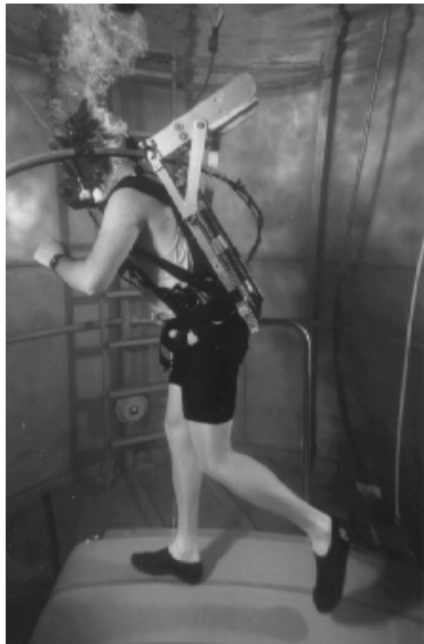
Figure 1: A test subject participating in a Mars-gravity simulation at NASA Ames Research Center exercises with a backpack load configured to emulate a proposed life support system [21].
